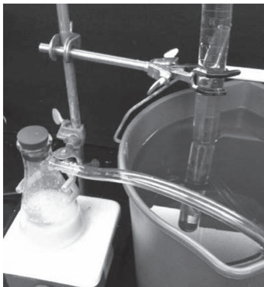
Figure 1: Arrangement for silver nanoparticle-baker's yeast biotoxicity experiment.
